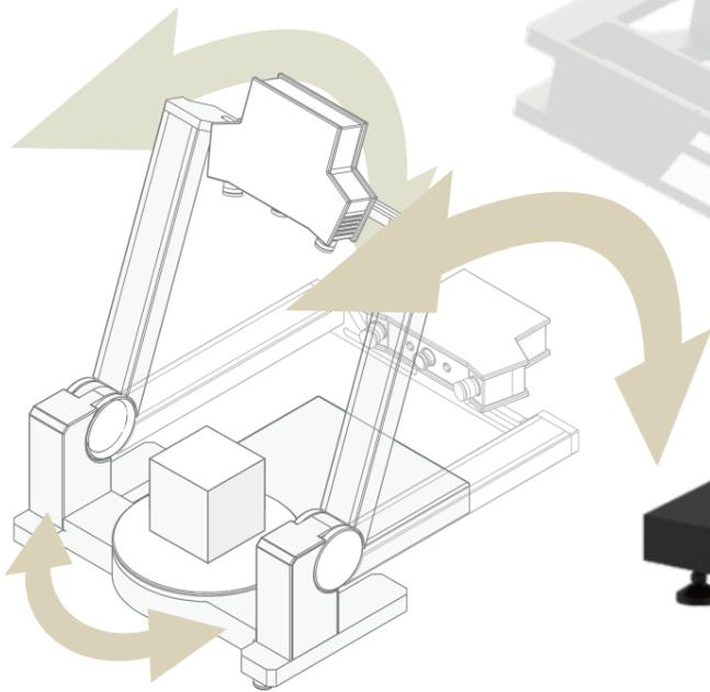
Conventional automatic systems require users to use jigs or clamps to hold down the objects, due to their swinging movement.
